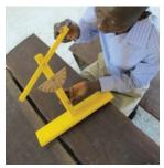
Loosely fix the balancing arm to the pillar with a nail.
