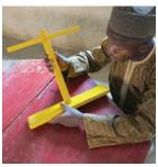
Loosely fix the balancing arm to the pillar with a nail.
