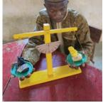
Put equal weights on both arms and the scale should balance level.
