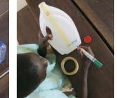
Pour 500ml into the 1l bottle. Mark '500ml' on the masking tape.
